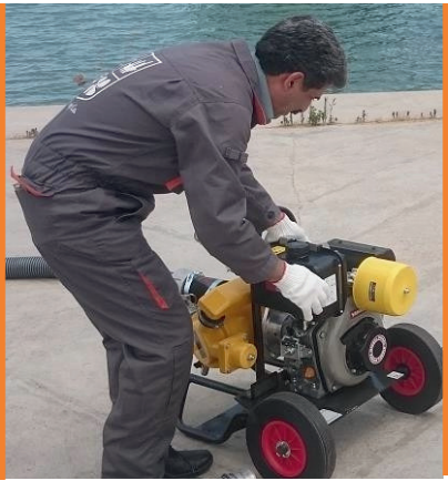
Diesel Driven Transfer Pump
